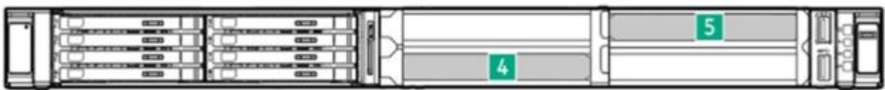
Front risers of GPU CTO server
